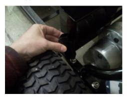
7. Repeat fixing of mudguard support on near side. **REMEMBER** Re tighten bolts on both sides after fixing.
