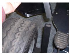
5. Drop mudguards on to support when required to height
