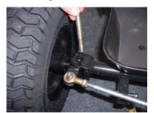
2.Remove washer from top of king pin as this is no longer required
