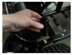
6.The rear mudguard supports are held in place using the same front motor bolt on either side of the cross support.
